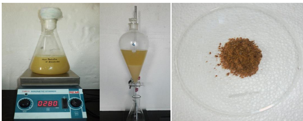
Fig. 4. Massproduction of biosurfactant from A. fumigatus (PN1) and extraction of biosurfactant by solvent extraction method
