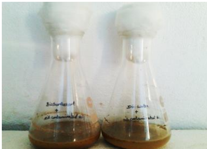
Fig. 6: Application of biosurfactant in motor oil removal from contaminated sand
